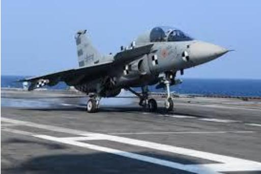
The fighter is undergoing additional carrier trials, following which it will return to the Shore Base Test Facility (SBTF) at Goa. **The flight represented a historic moment for Indian aviation, being the first time a locally-produced jet has arrested aboard a carrier. – “TEJAS”**
